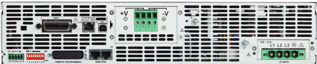
Rear panel with wire clamp connectors
