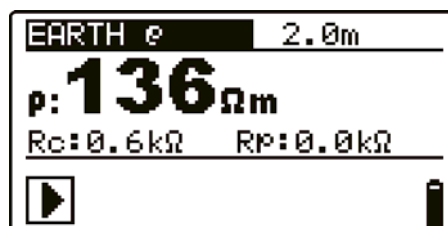
Figure 5.10: Example of specific earth resistance measurement result
