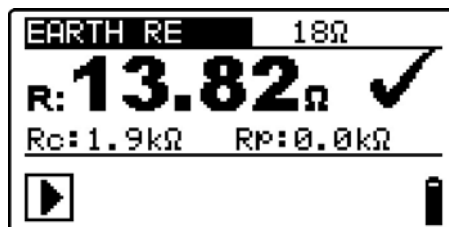
Figure 5.4: Example of earth resistance measurement result
