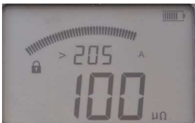
Min current during test was 205 A
