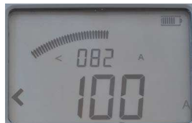
Picture shows that the test current was below 100 A.
