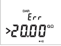
With the C.A 6532, if this occurs during a DAR or PI measurement, the instrument interrupts the measurement and displays the screen shown opposite.
