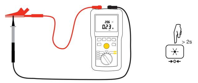
The display changes to zero and the  $\rightarrow 0$  + symbol is displayed. The resistance of the leads will be systematically subtracted from all continuity measurements. If the resistance of the leads is > 10  $\Omega$ , there is no compensation.
