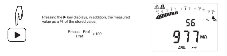
In insulation measurements, only the digital display is modified by the ∆REL. The bargraph continues to display the true measured value.
