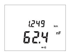
The instrument displays the capacitance and the corresponding line length, computed from the programmed capacitance per unit length.
