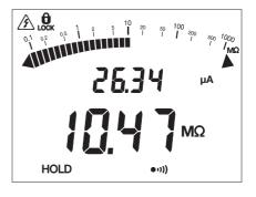
Then long-press the **MEM** key to store the measurement. The measurement is recorded in the first memory slot
