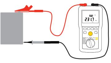
The instrument displays the voltage on the terminals. It detects whether the voltage is AC or DC and, if it is AC, the C.A 6532 also displays the frequency.
