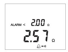
While it is displayed, you can change this value using the  $\blacktriangle$  key, except during insulation measurements. For each position of the switch, there are 3 pre-recorded threshold values:
