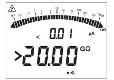
If, during an insulation measurement, the value to be measured exceeds the measurement range (which depends on the instrument and the test voltage), the instrument so reports.
