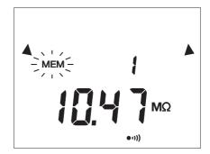
necessarily displayed at the time of storage: voltage, current, duration of tests T1 and T2 in the case of PI and DAR, etc. The bargraph indicates the level of filling of the memory.
