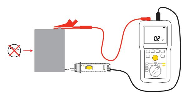
When the probe is connected, the  $\neg$  symbol is displayed.
