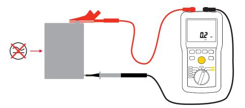
The measurement is displayed on the main display unit and on the bargraph.
