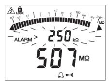
In the example above, the user can thus check that their continuity measurement is indeed less than 2  $\Omega$ , just by listening, without looking at the display unit. They can check insulation quality in the same way.
