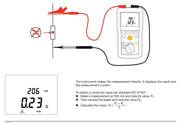
If an external voltage > 15 V appears during the continuity measurement, the instrument is protected without a fuse. The continuity measurement is stopped and the instrument reports an error until the voltage disappears.
