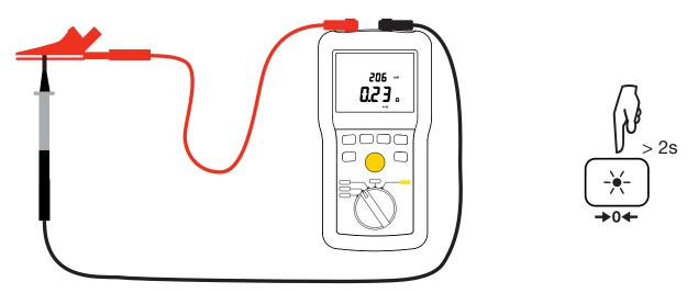
The display changes to zero and the  $\rightarrow_0 \leftarrow$  symbol is displayed. The resistance of the leads will be systematically subtracted from all continuity measurements. If the resistance of the leads is > 10  $\Omega$ , there is no compensation.
