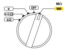
Set the switch to the  $M\Omega$  position.
