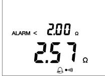
While it is displayed, you can change this value using the  $\blacktriangle$  key, except during insulation measurements. For each position of the switch, there are 3 pre-recorded threshold values:
