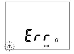
If, during a continuity or resistance measurement, the instrument detects an external voltage in excess of 15 V (AC or DC), it interrupts the measurement and displays the screen shown opposite.
