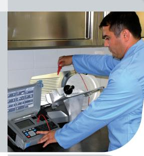
The MI 3310 25A SigmaGT is a multifunctional portable test instrument intended to perform all measurements for complete testing the electrical safety of portable electrical equipment. The instrument can operate from mains power or batteries.
