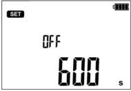
Use buttons ♠ and ♥ to set Auto-OFF time or to inactivate this function (horizontal lines – Auto-OFF function is inactive). Auto-OFF function is used to turn-off inactive meter after a preselected time.
