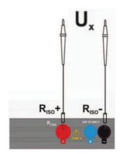
Connect the meter to a voltage source.
