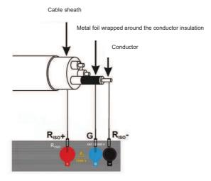
The same shall apply when measuring the resistance between two conductors of the cable, attaching to  ${\bf G}$  terminal other conductors that do not take part in the measurement.
